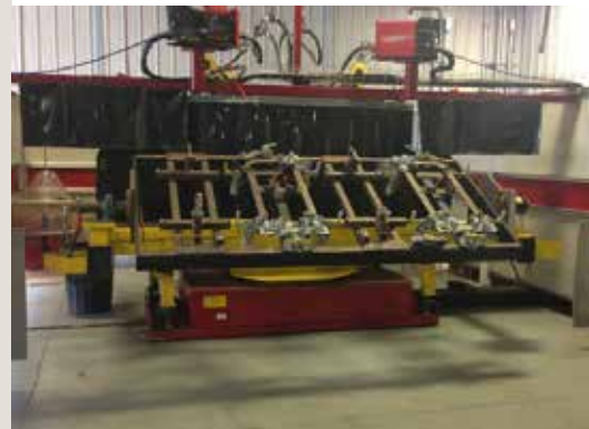
Custom fixtures and jigs are developed in-house to ensure repeatability in fabrication and delivery of quality products.
